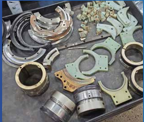
Items replaced in the slotting section during a typical asset management visit
