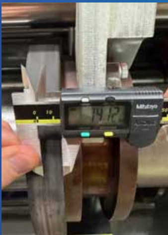
Checking the alignment of the scoring heads is a critical part of every asset management visit
