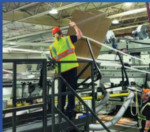
Adjusting folding rods for optimal box quality
