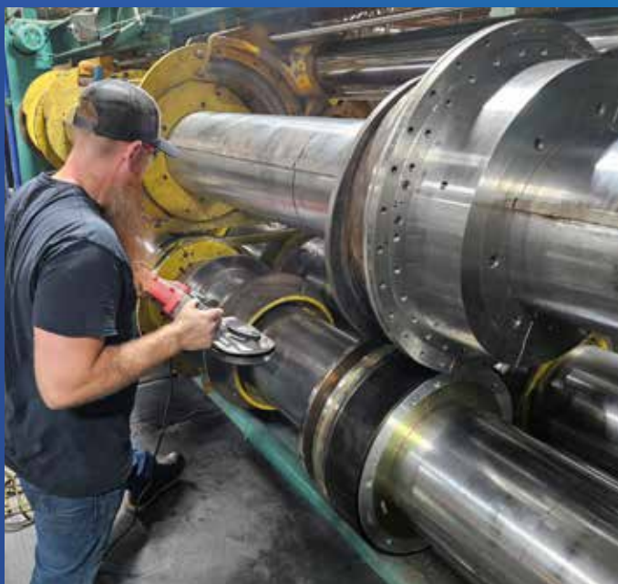
Sauer technicians removing solid heads from shafts to make room for split heads
