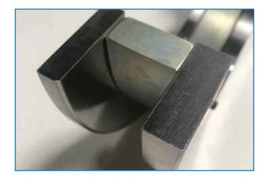
The Sauer System three-ring design consists of an inner wear plate, an outer wear plate, and yoke spacer. When the wear plates become worn, they can be flipped around, or replaced individually. Conversely, the OEM design is a one-piece "U-shape" that cannot be flipped and is expensive to replace.
