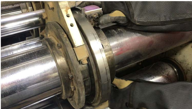
Checking head for lateral play
