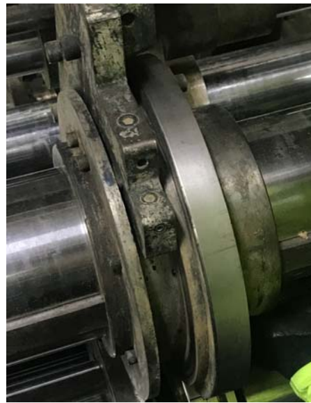
OEM Style yoke with carbide buttons
