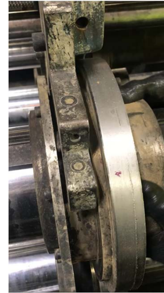
OEM Style yoke with carbide buttons
