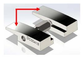
• Next, install the adjustable holder with the closed end of the knife facing up. Then slide up clearing entry slot area for next piece:
