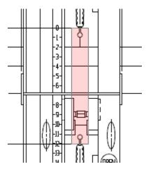
2) Position the rings laterally such that the widths between slots match the box dimensions and tighten them down by tightening the "OPEN" side screws. Note that "0" on the horizontal key corresponds to the center line of the cylinder. One ring will typically remain on "0" at all times, like a center slotter head on a flexo folder-gluer.
