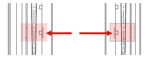
• First, install a clamp, with the tapers pointed down. The tapers are indicated by the arrows. Then slide up clearing entry slot area for next piece:
