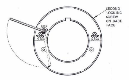
UNLOCK BOTH SIDES OF THE HEAD. Insert 3/16" Allen wrench in the locking screw and rotate in the opposite direction of the arrow approximately 1/2 turn.
