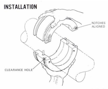
ASSEMBLE ON SHAFT. Hold the lower half of head (half with vertical pins) on the shaft and mate the top half. The retaining screw will fit into the mating clearance hole when parts are properly lined up.
