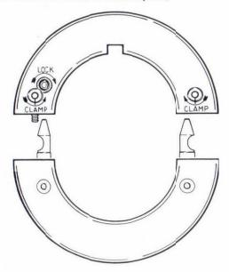
**SEPARATE THE HALVES.** The separated halves should be aid on their sides (faces) to insure that the vertical pins and retaining screw are not damaged.
