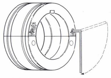
LOCATE ON SHAFT. Move the mated halves of the head to the desired position on the shaft. Insert the 3/16" Allen wrench into the clamp shaft farthest away from you and rotate in the direction of the arrow. (This can be done from either face.) The head is now clamped securely in position. (NOTE: Only one side of the head need be locked. The second locking screw can remain loose.)
