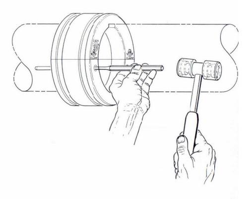
Emergency removal of the head can be accomplished without damage to the Kam-Lok device or the head itself. Simply remove the dowel pins from the lower half of the head as shown in the illustration above.
