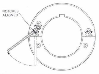
UNCLAMP BOTH SIDES OF THE HEAD. Insert the 3/16" Allen wrench in the clamp shaft and rotate in the opposite cirection of the arrow as far as it will turn. (The notches in the clamp shaft and casting will be aligned when the head is unclamped.)
