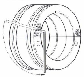
CLAMP THE SIDENEAREST YOU. Insert a 3/16" Allen wrench into clamping snaft and rotate in the direction of the arrow until tight.
