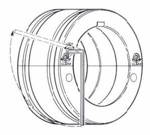
LOCK THE SIDE NEAREST YOU. Insert the 3/16" Allen wrench in the locking screw and rotate in the direction of the arrow until tight.
