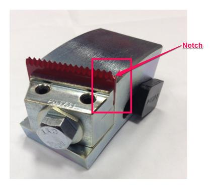
4) Jog the upper slotting shaft around one time and ensure the notch on the tab knife just "kisses" the 3/32" (thin) blade on the lower glue tab cutting head. If the knife "misses" the blade, loosen the clamp block and use the jacking screws to raise the block until the correct contact is made. Both screws should be tightened the same amount, 1/4 turn at a time.
