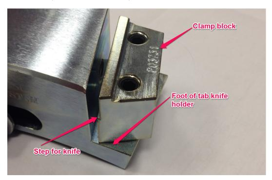
3) Ensure the knife is mounted such that the notch is flush with the edge of the holder and therefore butts up to the male slotting blade.
