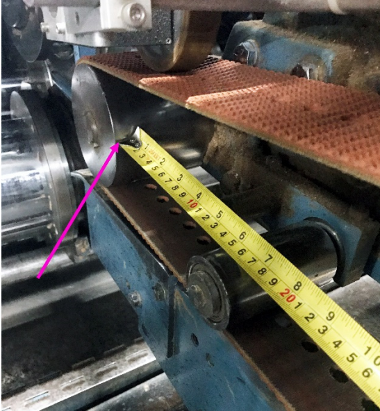
Adjustable roller measurement starting point
